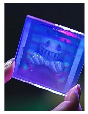
Hologram observed by transmission via halogen spot, after bleach. When the hologram is successful, this image will be very strong.
