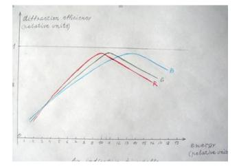
Figure 2. An example Diffraction efficiency according exposure, for a test batch of U08C, measured by Vladimir.
