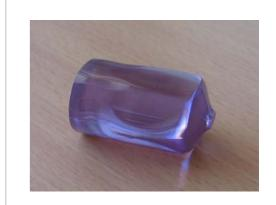
AOTK uses the advance Czochralski method technology to grow Nd:GdVO<sub>4</sub> crystal. The crystal is tetragonal which means that there are two equivalent "a" directions and a "c" direction, all mutually orthogonal. A typical laser rod is oriented with the rod axis along an a-axis of the crystal. Maximum absorption of pump light occurs for polarization along the c-axis.
