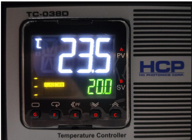
Fig. 1.2.1 The front panel of TC-038D controller, the function of A to G has been listed below
